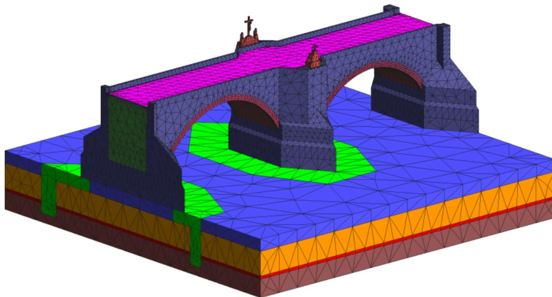
Finite element mesh (20,409 nodes; 97,004 linear tetrahedra)
