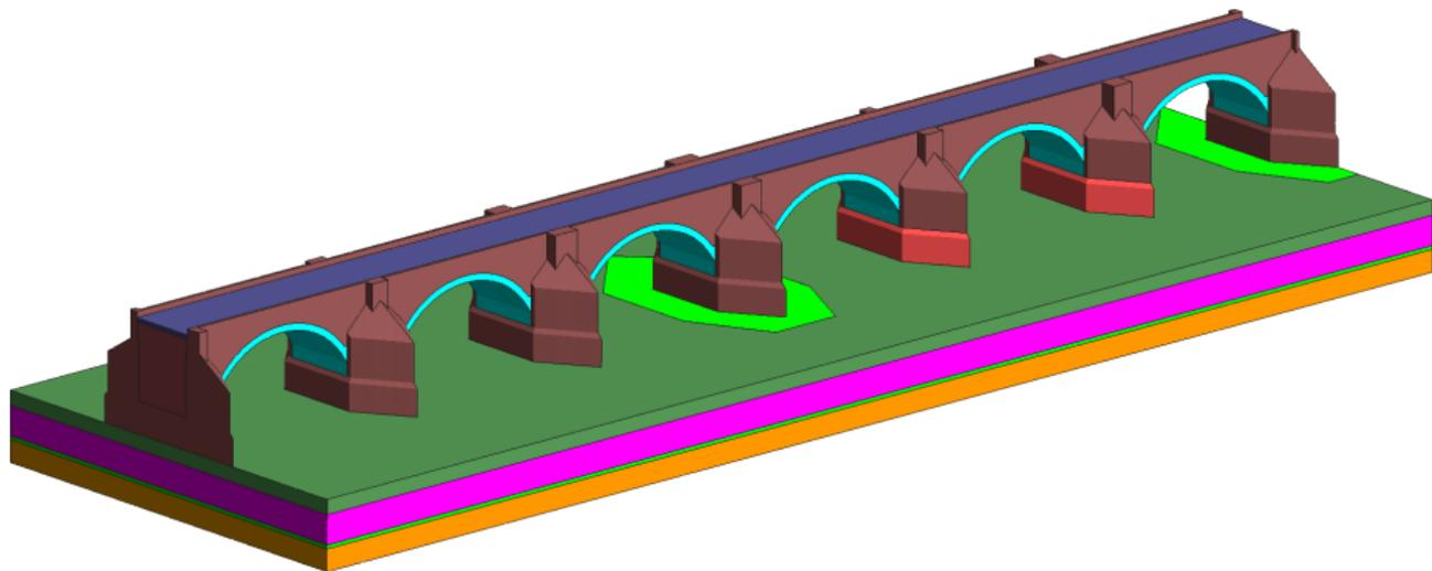
Six-span model (31,725 nodes, 142,976 linear tetrahedra)
